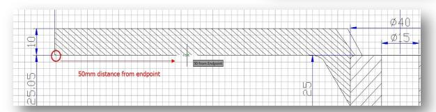
And within Object Snap tab, you can find a new added option called *Divide Segments*. This option allows snap the divided segment points of objects like line, arc, spline, pline, ellipse arc, mline and any other lines. Before, if you want to find the divide point, first you need to generate the divided points object, then snap those points to draw. Now as long as you pass the cursor over an object mentioned above, you will see a green snap point at accurate distance.
