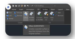
You can **Offset the surface in one direction** (the arrows will show on one side of the surface) by entering a distance or select the point on the drawing.
