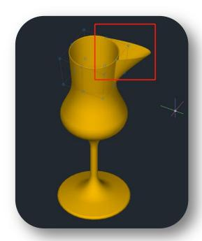
REMOVE: Removes control vertices. There are at least 2 control vertices in each direction.
