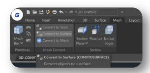
**Eligible objects include:** 2D solids, 3D solids, Mesh objects, Planar 3D faces, Regions, Zero-width polylines with thickness, Polylines with global-width, Lines with thickness, Arcs with thickness, Closed plane curve.
