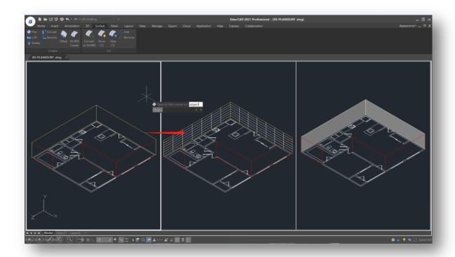
SURFU / SURFV: System variable, sets the number of lines displayed on the surface
