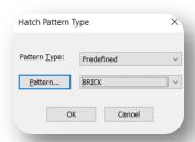
• Pattern name: Displays a selection of ANSI, ISO, and other industry-standard hatch patterns. The Pattern option is not available when Type is set to User-defined.
