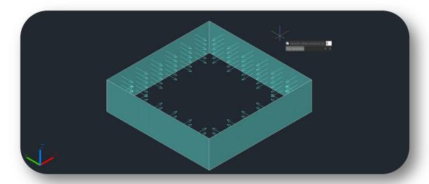
If you type "Both sides", you can Offset the surface in both directions (the arrows will show on both sides of the surfaces)
