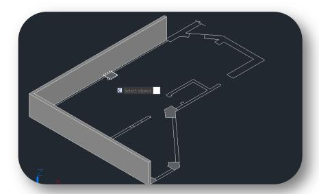
**PSOLWIDTH**: System variable, sets the default width for the 3D polysolid. **PSOLHEIGHT**: System variable, sets the default height for the 3D polysolid.
