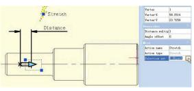
**3. Test dynamic block**: Exit from block editor, drag stretch grip to stretch the keyway, as shown in the picture.
