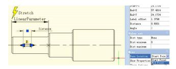
**3.Add the stretch rightwards action for the keyway and realize chain action:** Select the "Distance" linear parameter and modify the chain action of prosperity from "NO" to "Yes" as the following picture shows:
