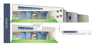
The boundary can be a polyline, a rectangle, or a polygon whose vertexes are limited within the global scope of the underlay. You can modify the boundary of the graphics to be clipped. When you clip the graphics, you do not change the object in the external reference or block, but only change the way they are displayed.
