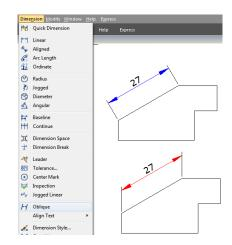
Remark: To align the oblique angle if you don't know the exact measurement, use snaps to pick two points on the entity.
