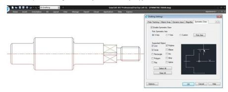
In GstarCAD 2020, it is possible to directly draw symmetrical shapes with Symmetric Draw tool. When drawing the first half you get another half automatically. The default symmetry axis is X-axis, but user can specify Y-axis or any line in the drawing as symmetry axis reference.
