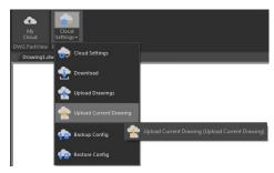
After finish drawing modifications, if you check the option *Automatically upload a drawing when you save* on *Drawing transmission settings*, and then *Save* or either press the *Upload Current Drawing* button in the ribbon to upload your modified drawing to the cloud.
