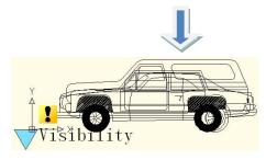
**5. Test Dynamic Block**: Insert the edited Dynamic Block into a drawing, select Dynamic Block and click the grip of Visibility Parameter, choose one item in the pop-up pull-down list, Dynamic Block will change the display state automatically, as shown in the following picture.
