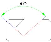
To dimension an angle encompassed by an arc:
