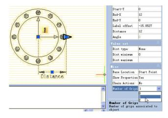
**3. Add Action:** Click the Scale icon on the Action Panel, appoint parameter for Action and box the whole access hole as Action Object, as shown in the following picture.
