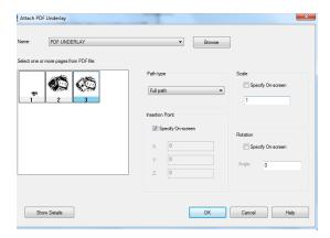
After inserting the PDF file as underlay, Then you can start drawing or placing geometry at specific point of the underlay.
