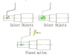
**4. Test dynamic block**:Insert the dynamic block, drag the blue grip, then move the keyway to the right accordingly, as shown in below picture. Obviously, the dynamic block can achieve the expected results. Please pay attention, if it is not run with ortho constraint, the keyway can move towards every direction because the direction of the
