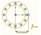
Exit from Block Editor, Drag the grips of the Access hole Block again, you can see, that after the change from Linear Parameter to Polar Parameter, we can drag the grip to scale the dynamic block in any direction.
