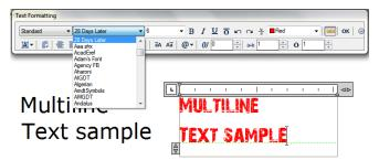
Justify Multiline Text: You can specify the attachment point at the top left, top center, top right, middle left, middle center, middle right, bottom left, bottom center, or bottom right. The multiline text can flow left to right, right to left, top to bottom, or bottom to top.
