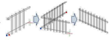
Enter into Block Editor, Stretch, the ways of adding Array Action as in the following picture, the bold object expresses the relevance with the selected action. The Polar Parameter determines the way of Array directly, the Polar Array will regard the direction of the Polar Parameter as Array direction, achieving Array functions in any direction.
