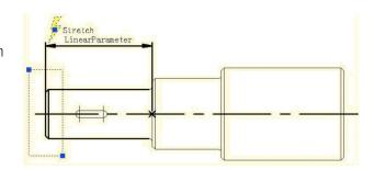
**2.** Add Move Action for keyway: Select the left grip of the linear parameter when moving, stretching the related parameter points. Move the objects of action and select the whole keyway, as in the following picture.
