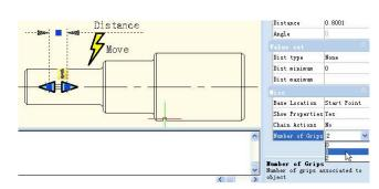
Save and exit the Block Editor, choose the Dynamic Block, you will find that one grip has disappeared. In fact, after changing the number of grips from "2" to "1", the first thing that disappeared was the basic grip of parameters, namely the first point when adding parameters.
