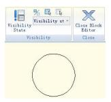
**2.** Add base point: Click "base point" parameter on the parameter panel, put the parameter on the center of the circle according to system prompt, as shown in the below illustration.
