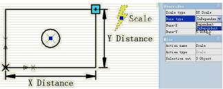
Specify new base: Single click the right input box of "Base-X" and "Base-Y", you can manually input the coordinate value or you can single click the small button with ellipsis dots on the right of the input box and snap the base point, as shown:
