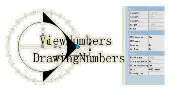
**3.** Add rotate action: Click the rotation action button on the action panel, match parameter, object and position for the action and select the whole index symbol as the object of the action.
