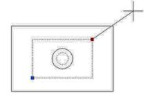
**6. Scale Type:** There is "Scale Type" in the Scale Action Properties. The default value is "XY Scale". If you choose "XY Scale", the dynamic block scales whenever the scale grip moves to X axis or Y axis. If you choose "X Scale", it scales only when the grip of the scale moves to X axis. Same, when you choose "Y Scale".
