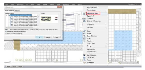
The objects that you select from the selected xref or block are temporarily extracted and made available for editing in the current drawing. The set of extracted objects is called the working set, which can be modified and then saved back to update the xref or block definition.
