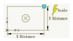
**3. Test the Dynamic Block**: After exiting the Block Editor, drag the grip of the top right corner of the rectangle, you can see the whole dynamic block is scaling as the grip is moving. It is easy to find that both the circle and the rectangle scale by the base point of the XY Parameter.
