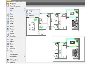
Xrefs can be nested in another xref and attached to current drawing. In the process of attaching, you can select insertion position, scaling factor and rotation angle for xrefs.
