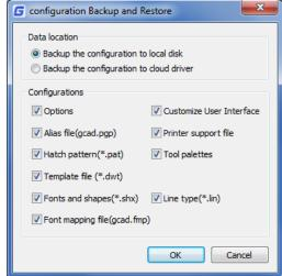
You can also restore settings by clicking the *Restore Config* button on the ribbon. Select *Yes* button to check and save the current configuration before restore it.
