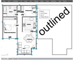
For example, use this tool extract the outline shape of a floor plant house to later calculate its total area or to reference draw the roof of it.
