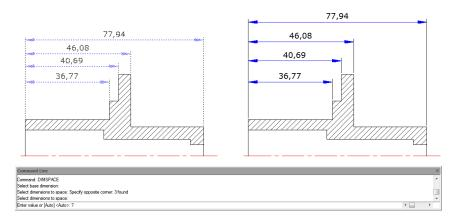
original space is not equal values. If you set the space value to 0 when adjusting space among dimensions, you can align selected dimensions at the dimension line as well.
