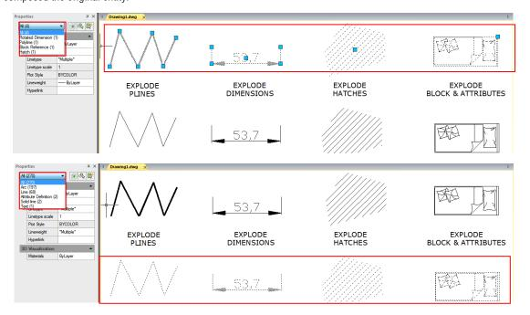
With the following exceptions, exploding an entity usually has no visible effect on a drawing:
