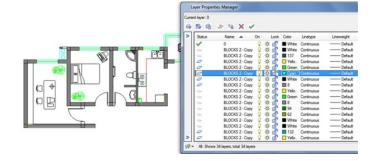
through XDWGFADECTL variable. In addition you can control Xref layer properties directly into the Layer Manager Properties dialog box.
