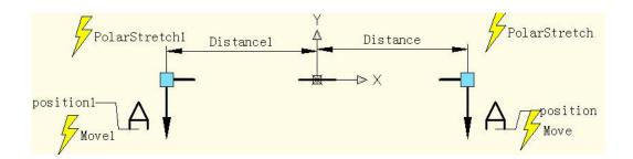
**4. Test Dynamic Block:** Open the graphic which needs to be dimensioned and insert the completed dynamic block (Fig 4.1).
